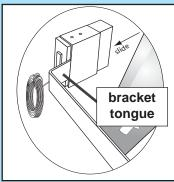
FIG. 4-3 Attach Safe-T-Beam® to brackets
